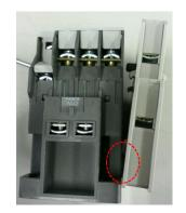
Match hooks on UR-02 with grooves on the side of a MC
